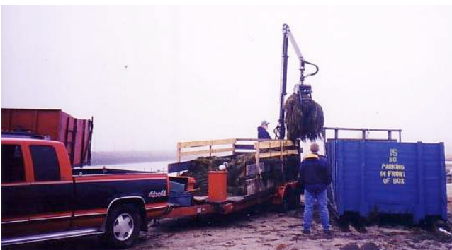
Fig. 22: Alternative methods of unloading the daily Ascophyllum nodosum harvest with mobile equipment in southwestern NS.
