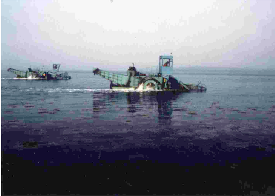
Fig. 11: Harvesting of Ascophyllum nodosum with mechanical Aquamarine harvesters from Scotia Marine Products Ltd. in southwest NS. (photography by J. Pringle).
